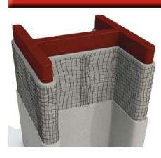
At mesh joints, an overlap must be introduced according to certification rules. If the overlapping mesh is not correctly installed with adequate adhesion, the upper layer of mesh will lift. This will cause project delay due to rework of the mesh and the subsequent coats.
