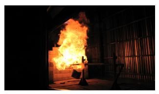
Jet fires are regarded as one of the most significant hazards in the Oil, Gas and Energy industries due to resulting rapid steel temperature rise, highly erosive nature of the flame and risk of rapid incident escalation.
